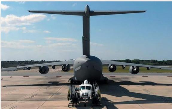
**IMAGE 3: Rapid Deployability.** Disassembly and reassembly of the MC-208 Guardian for C-17 transport can be done in 13 hours with only 5 crew, putting the aircraft on the ground and mission-ready almost anywhere in the world within 48 hours. Two disassembled aircraft fit on a C-17.
