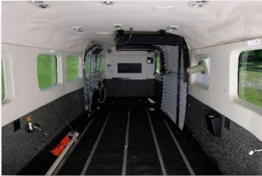
**IMAGE 5: MEDEVAC/CASEVAC.** A significant added advantage of the MC-208 Guardian is its cargo capacity and its ability to perform medical and casualty evacuations, as well as airdrops of personnel or supplies via an air-operable roll up door.
